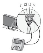
Verify the absence of voltage in L1, L2 and L3 to PE at the AC terminal.
