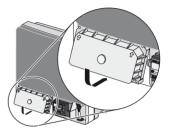
Pre-screw all four screws of the DC lid and then tighten them (torque: 3.5 Nm).
