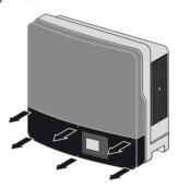
To remove the lower enclosure lid, lift it up from the bottom.
