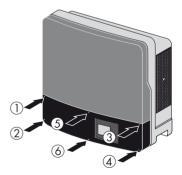
9. Plug the Electronic Solar Switch in firmly right up to the stop.
