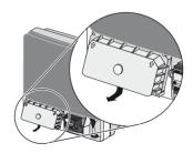
4. Remove all surge arresters from the slots. To do this, compress the grooved areas on either side.
