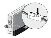
Remove the fan and clean it with a soft brush, a paint brush or a cloth and water.
