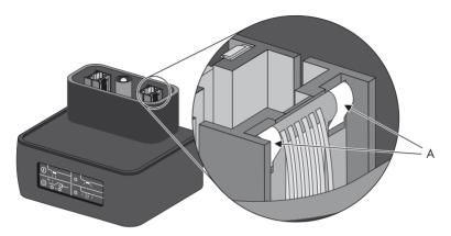
If the metal tongues are discoloured or burnt right through (B), the Electronic Solar Switch can no longer perform reliable disconnection of the DC side.
