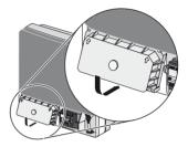
6. Pre-screw all four screws of the DC lid and then tighten them (torque: 3.5 Nm).
