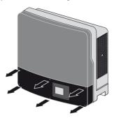
To remove the lower enclosure lid, lift it from the bottom.
