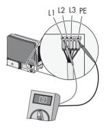
9. Verify the absence of voltage in the multi-function relay to PE at all terminals.
