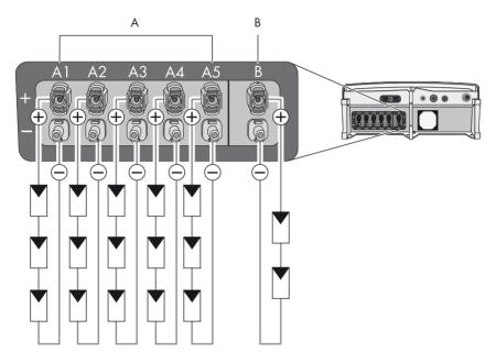
Up to four strings (Sunny Tripower 10000TL / 12000TL) or five strings (Sunny Tripower 15000TL / 17000TL) can be connected at input area A. One string can be connected at input area B.
