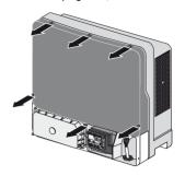
4. Pre-screw the transport lid of the replacement device with the six enclosure lid screws and corresponding conical spring washers to your original inverter and then screw down tight in the sequence shown on the right (torque: 6.0 Nm). The toothing of the conical spring washers must point towards the enclosure lid. This ensures proper earthing of the enclosure lid.
