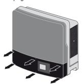
To remove the lower enclosure lid, lift it from the bottom
