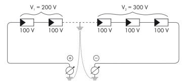
In this case, the earth fault is between the second and third PV modules.
