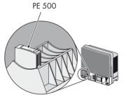
If surge arresters are only required for input A, the two surge arresters must be mounted on the two upper slots.
